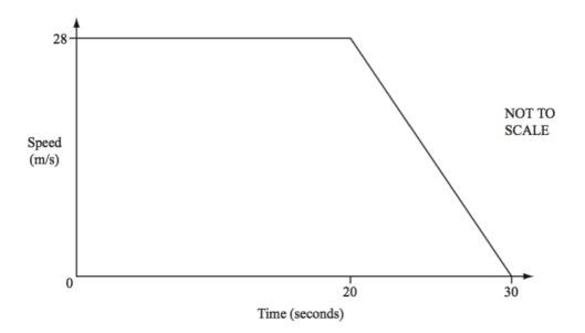
The diagram shows the speed-time graph of a car. It travels at 28 m/s for 20 seconds and then decelerates until it stops after a further 10 seconds.
