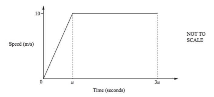
A car starts from rest and accelerates for u seconds until it reaches a speed of 10 m/s. The car then travels at 10 m/s for 2u seconds. The diagram shows the speed-time graph for this journey.
